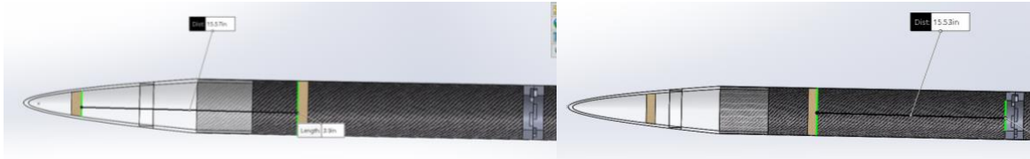
Figure 4.1.3: The Main Parachute Storage Section is ~15" (left); Avionics Bay Section is ~15.5" (right)
