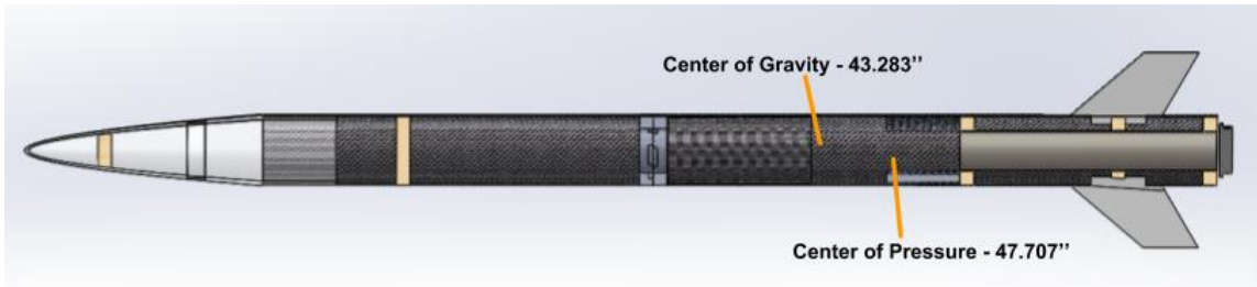
Figure 2.1.2: Cross Section Side View of Rocket with CP and CG indicated
