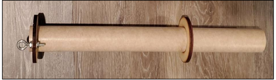
Figure 13-8: Centering Rings Fitted on Motor Mount Tube
