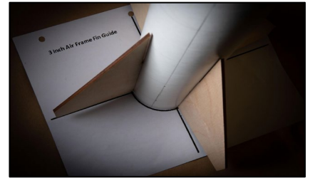
Figure 13-29: Align Each Fin to Crosshair Lines
