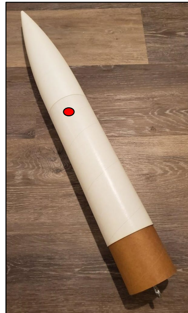
Figure 13-24: Nose Cone Fitted on Sustainer, Red Dot Indicates Drill Mark
