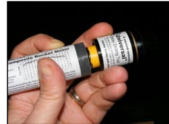
Figure 14-5: Removing seconds from delay
