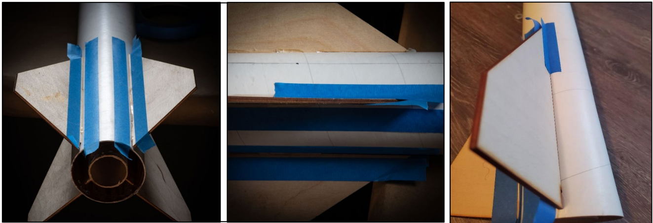
Figure 13-35 (Left); Tape Locations for Epoxy Fillets (Center); Dam Locations Right)
