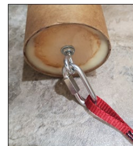
Figure 14:11: Parachute and Protectors Attached Inside of Quicklinks (Top); Quicklink Attached to Rocket and Closed (Bottom)
