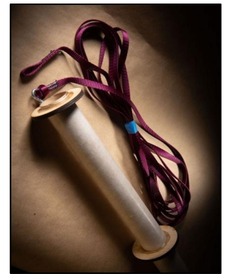
Figure 13-20: Shock Cord Attached to Eyebolt
