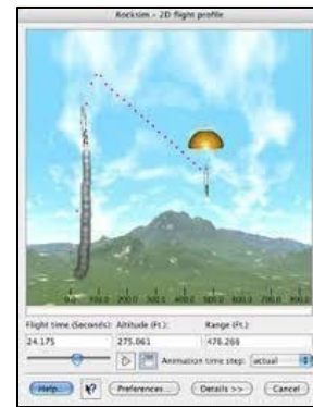
Figure 8-7: Parachute Selection with Simulation Data
