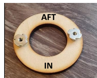
Figure 13-4: Aft Centering Ring with T-Nuts Installed
