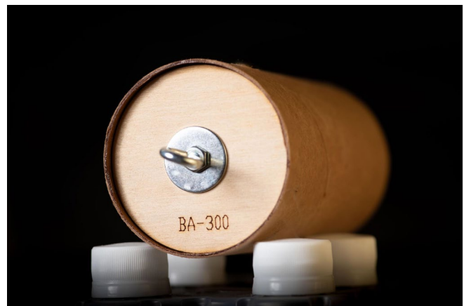
Figure 13-17: Bulkplate Installed in Coupler (Top); Applying Epoxy around Inside of Coupler (Middle); Bulkplate Installed in Coupler (Bottom)
