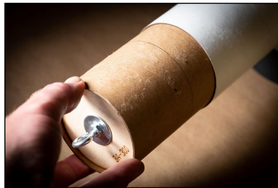
Figure 13-18: Example of Where to Draw Line on Coupler (Top); Epoxy Application (Middle); Coupler Placement (Bottom)
