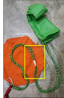
Figure 14-12: "Reef" the Shroud Lines Using Tape
