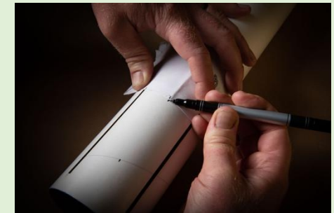
Figure 13-38: Rail Button Alignment on Launch Rail (Top); Marking an 'X' on the Vertical Line Where the Line Intersects with the Aft and Forward Centering Ring (Bottom)
