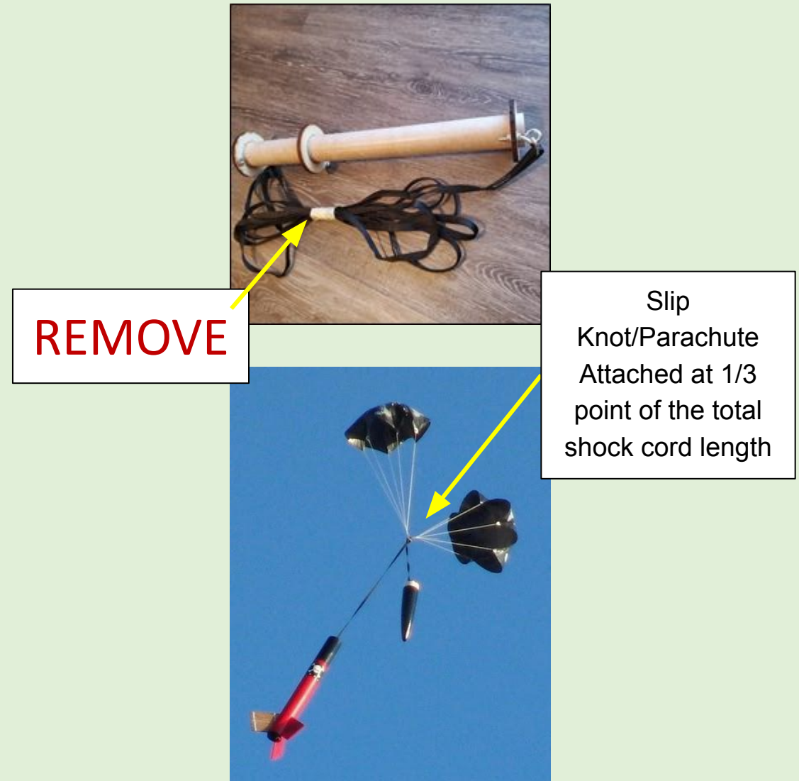
Figure 13-40: Masking Tape and Shock Cord (Top); Knot Location on Shock Cord (Bottom)
