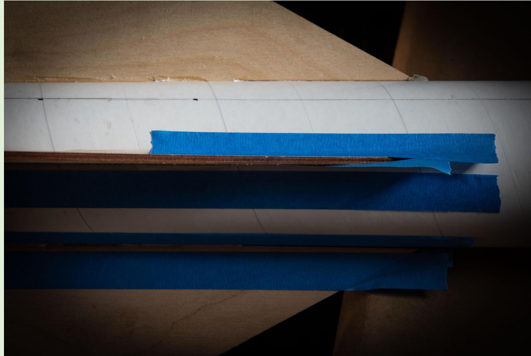
Figure 13-35: Tape Locations for Epoxy Fillets (Left, Center); Dam Locations (Right)
