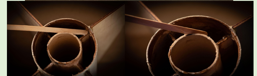
Figure 13-37: Slide Aft Ring to Fins (Top); Epoxy Outside of MMT (Left Middle); Epoxy Inside of Airframe (Right Middle)
