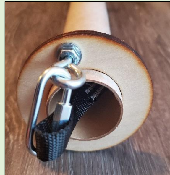
Figure 13-21: Shock Cord Installed Inside Motor Mount Tube Using Eyebolt (Left) and Quicklink and Eyebolt (Right)
