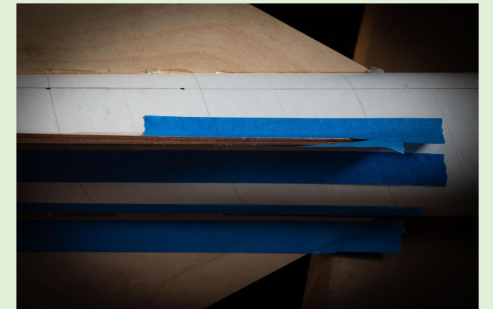
Figures 13-34, 13-35: Tape and Dam Diagram; (Top Left); Tape Locations for Epoxy Fillets (Top Right, Center); Dam Locations (Bottom Right)
