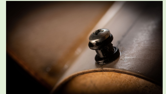
Figure 13-26: Rail Buttons are Drilled into the Mid-Centering Ring (Top) and Aft-Centering Ring (Bottom)
