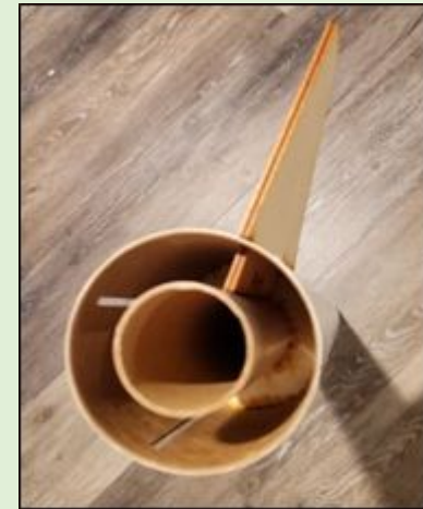
Figure 13-30: Tang Example (Top); Apply Epoxy to Tang (Center); Insert Tang in Fin Slot (Bottom)
