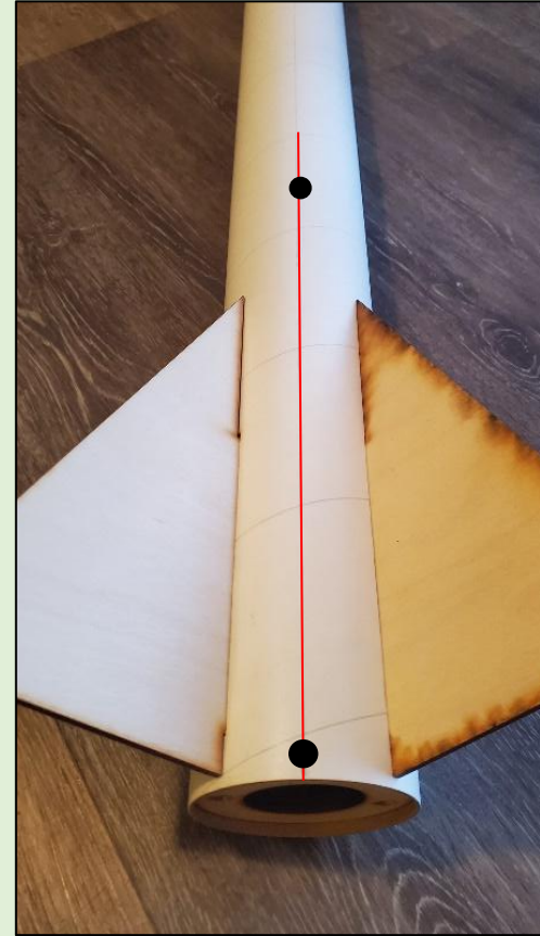
Figure 13-25: Markers to Indicate Rail Button Placement/Alignment (Bottom)
