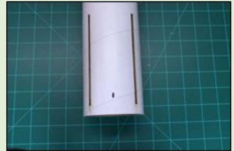
Figure 13-25: Drawing a Line at the Half Way Mark on Tape(Top); Drawing the Half Way Mark on the Air Frame (Bottom)
