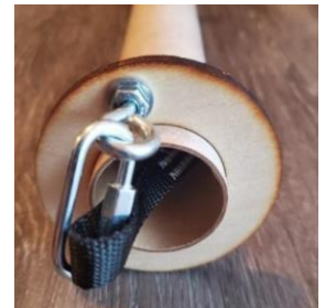
Figure 13-20: Shock Cord Attached to Eyebolt
