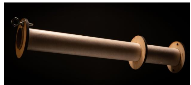
Figure 13-16: Epoxy Eyebolt Thread and T-Nuts (Top); Complete Motor Mount Assembly (Bottom)
