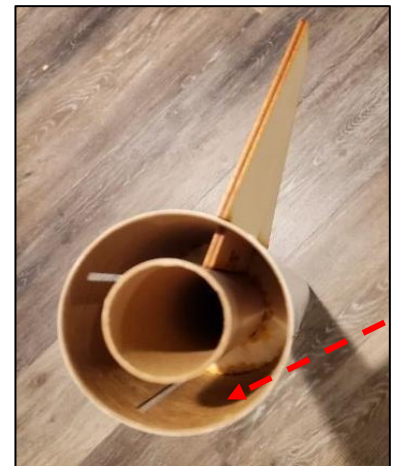
Figure 13-30: Tang Example (Top); Apply Epoxy to Tang (Center); Insert Tang in Fin Slot (Bottom)
