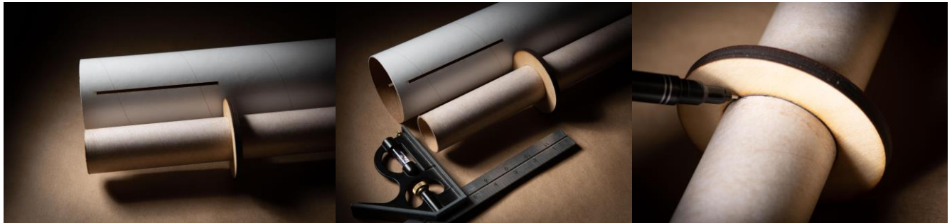
Figure 13-10: Center Motor Mount Ring Located above Fin Slot (Left); Measure the Length of the Fin Slot for Accuracy (Center); Draw a Line on the Motor Mount Tube around the Center Motor Mount Ring (Right)
