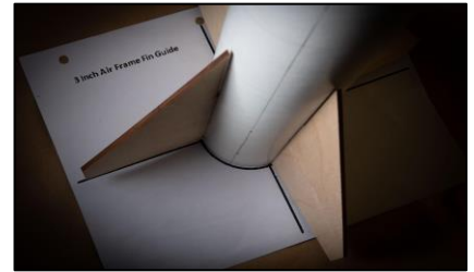
Figure 13-29: Align Each Fin to Crosshair Lines
