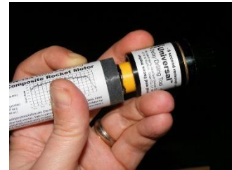
Figure 14-5: Removing seconds from delay
