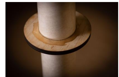
Figure 13-15: Motor Mount Placement with Line (Top); Applying Epoxy to the Mid-Centering Ring (Center); Completed Mid-Centering Ring (Bottom)
