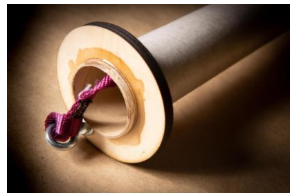
Figure 13-20: Shock Cord Attached to Eyebolt
