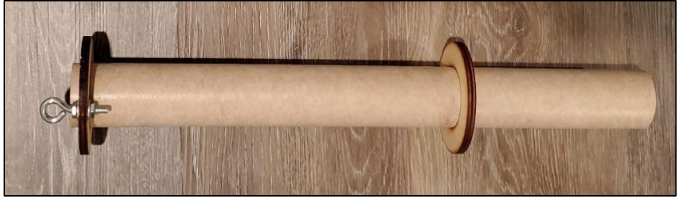
Figure 13-8: Centering Rings Fitted on Motor Mount Tube
