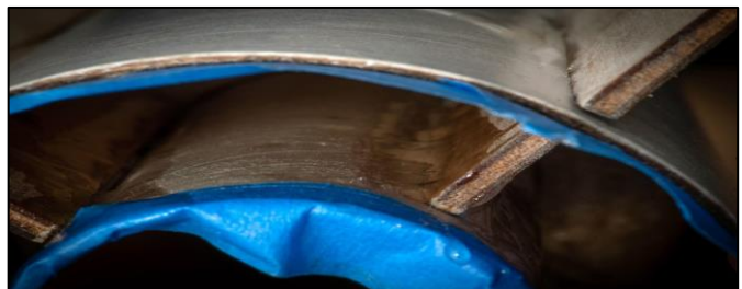
Figure 13-33: Fully Applied Epoxy Fillet between Motor Mount and Fin
