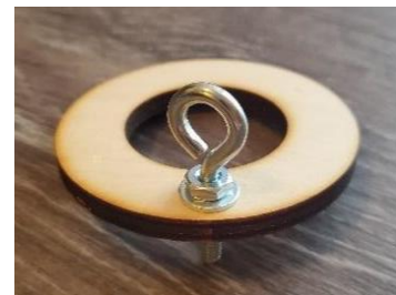
Figure 13-3: Forward Centering Ring with Eyebolt Installed
