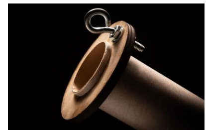
Figure 13-15: Motor Mount Placement with Line (Top); Applying Epoxy to the Mid-Centering Ring (Center); Completed Mid-Centering Ring (Bottom)
