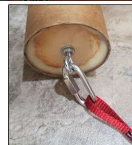
Figure 14-11: Parachute and Protectors Attached Inside of Quicklinks
