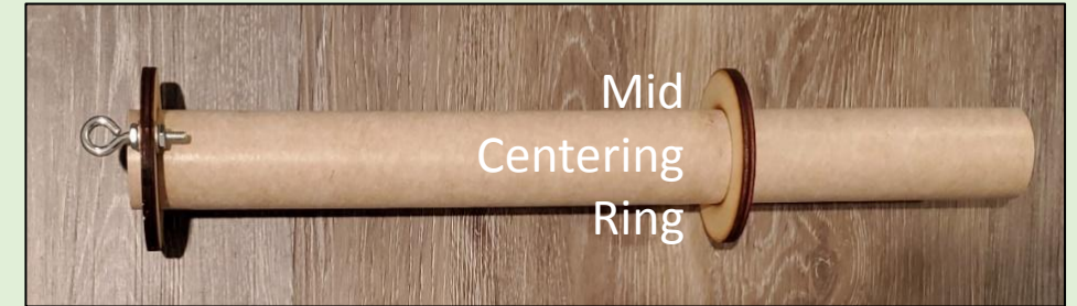
Figure 13-8: Centering Rings Fitted on Motor Mount Tube
