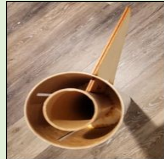
Figure 13-30: Tang Example (Top); Apply Epoxy to Tang (Center); Insert Tang in Fin Slot (Bottom)
