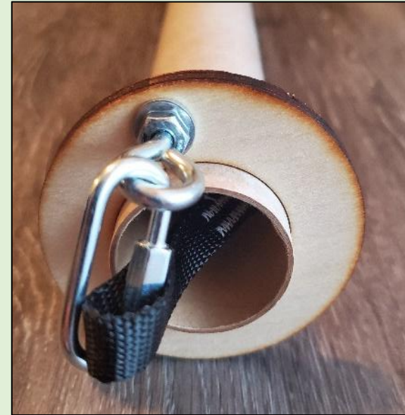
Figure 13-21: Shock Cord Installed Inside Motor Mount Tube Using Eyebolt (Left) and Quicklink and Eyebolt (Right)
