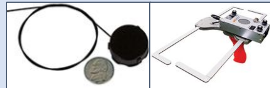
Figure 14-14: RF Tracking Device (Left); Yagi Antenna (Right)
