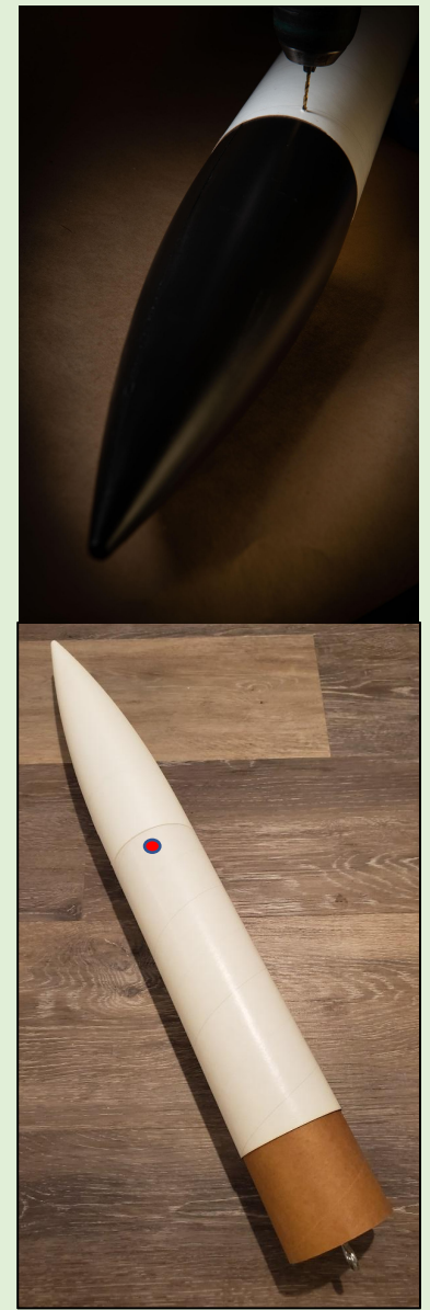
Figure 13-23: Drilling the Airframe and Nose Cone (Left); Figure 13-24: Nose Cone Fitted on Sustainer, Red Dot Indicates Drill Mark
