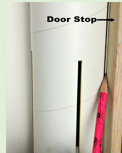
Figure 13-25: Markers to Indicate Rail Button Placement/Alignment (Bottom)
