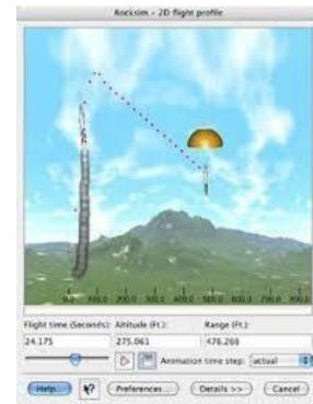
Figure 8-7: Parachute Selection with Simulation Data
