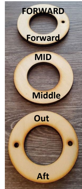
13-2: Aligned Centering Rings (top – Forward,
