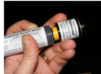
Figure 14-5: Removing seconds from delay
