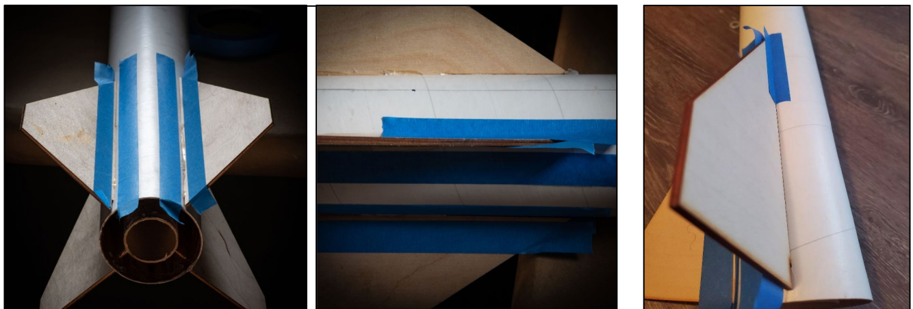
Figure 13-35 (Left); Tape Locations for Epoxy Fillets (Center); Dam Locations Right)
