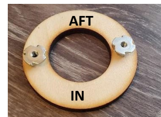
Figure 13-4a: Aft ring with T-Nuts
