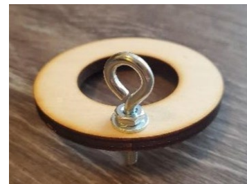
Figure 13-3: Forward Centering Ring with Eyebolt Installed
