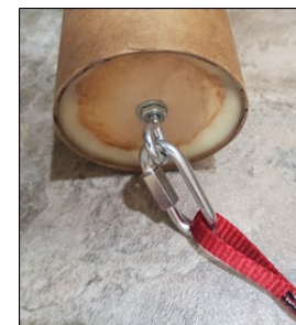
Figure 14-11: Parachute and Protectors Attached Inside of Quicklinks
