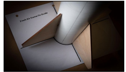
Figure 13-29: Align Each Fin to Crosshair Lines
