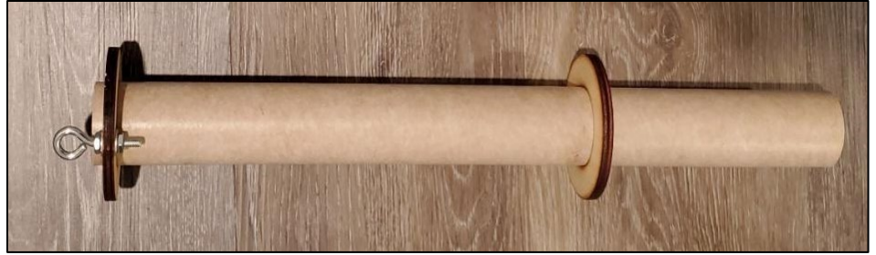
Figure 13-8: Centering Rings Fitted on Motor Mount Tube
