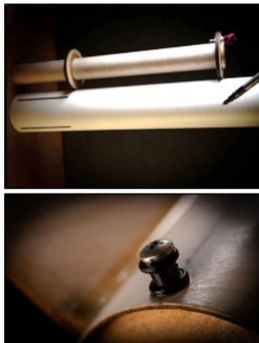
Figure 13-26: Rail Buttons are Drilled into the Mid-Centering Ring (Top) and Aft-Centering Ring (Bottom)
