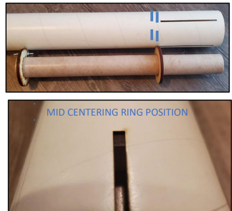
Figure 13-22: Relative Position of MMT Assembly Once Installed in Airframe (Top); Mid Centering Ring Should Sit Forward of Fin Slots (Bottom)
