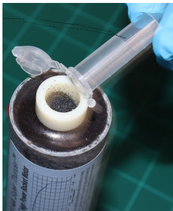
Figure 14-8: Pour Black Powder into Deployment Well
