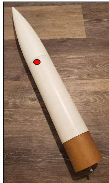
Figure 13-24: Red Dot indicates mark for drilling through airframe and nosecone
