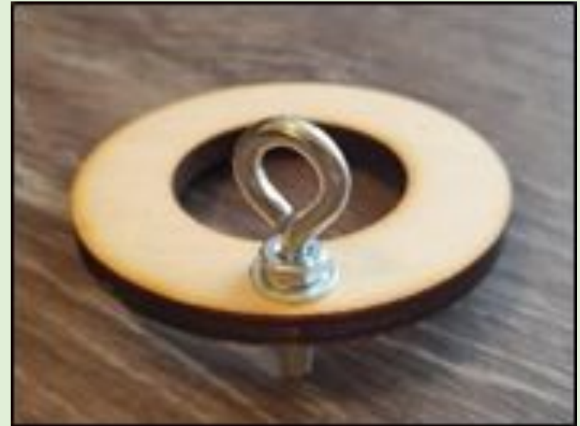
Figure 13-3: Forward Centering Ring with Eyebolt Installed
