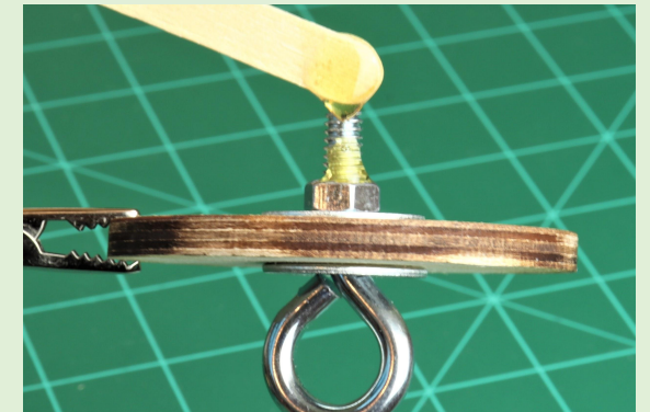
Figure 13-17: Dabbing epoxy on threads and nut of eyebolt
