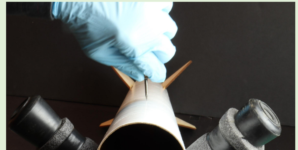
Figure 13-28: Drilling Vent Hole in Booster Section to Not Interfere with Rail Buttons Alignment (Left); Drilling Vent Hole in Sustainer Section (Right)
