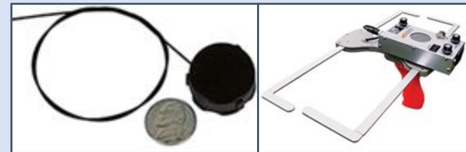
Figure 14-14: RF Tracking Device (Left); Yagi Antenna (Right)
