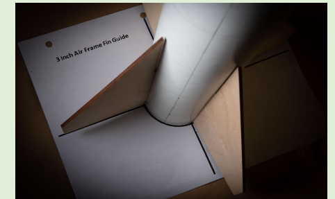
Figure 13-29: Align Each Fin to Crosshair Lines
