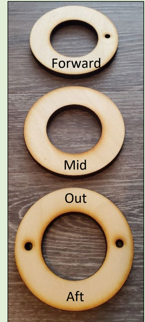
Figure 13-2: Aligned Centering Rings
