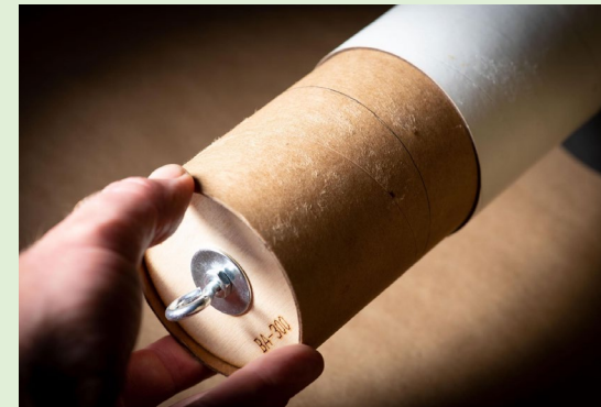
Figure 13-18: Epoxy Application (Top));Coupler Placement (Bottom)
