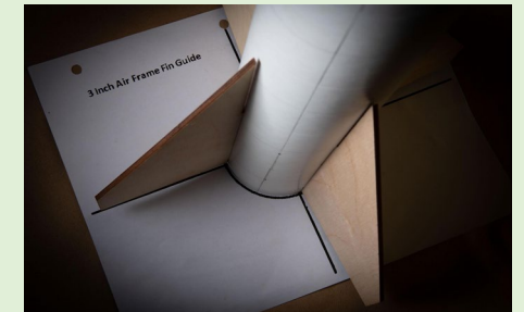
Figure 13-29: Align Each Fin to Crosshair Lines
