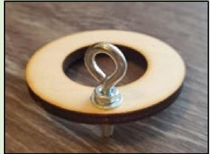
Figure 13-3: Forward Centering Ring with Eyebolt Installed
