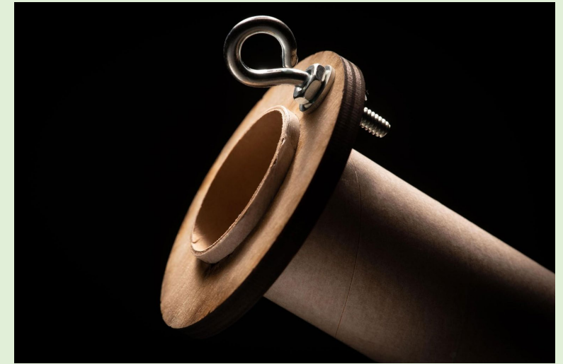
Figure 13-16: Epoxy Eyebolt Thread
