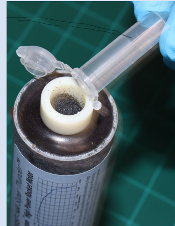
Figure 14-8: Pour Black Powder into Deployment Well
