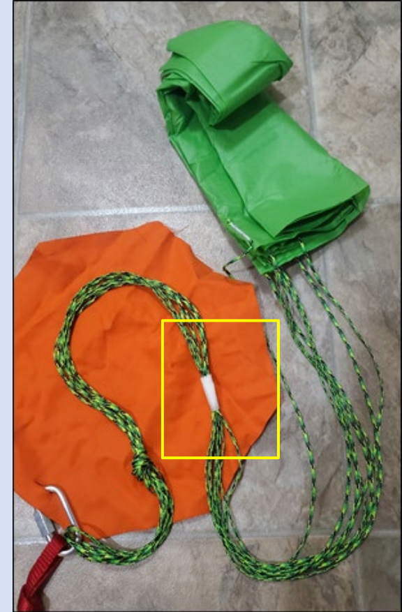
Figure 14-12: "Reef" the Shroud Lines Using Tape
