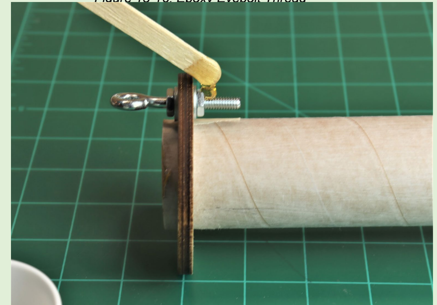
Figure 13-16: Epoxy Eyebolt Thread
