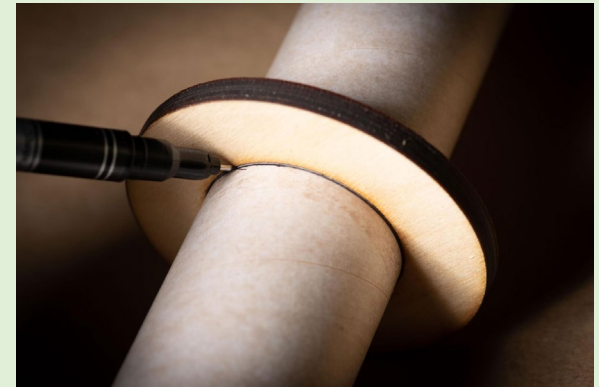
Figure 13-10: Center Motor Mount Ring Located above Fin Slot (Left); Measure the Length of the Fin Slot for Accuracy (Center); Draw a Line on the Motor Mount Tube around the Center Motor Mount Ring (Right)
