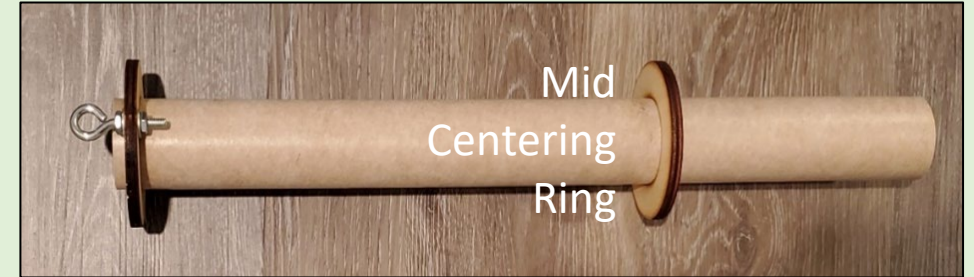
Figure 13-8: Centering Rings Fitted on Motor Mount Tube
