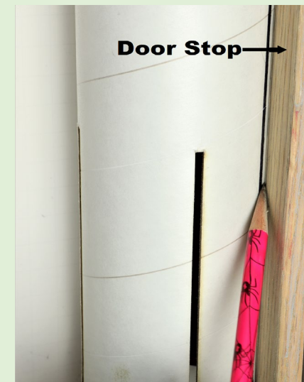
Figure 13-25: Markers to Indicate Rail Button Placement/Alignment (Bottom)
