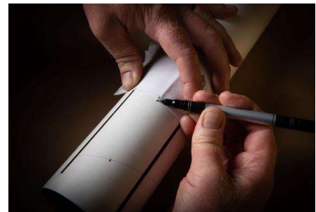
Figure 13-38: Rail Button Alignment on Launch Rail (Top); Marking an 'X' on the Vertical Line Where the Line Intersects with the Aft and Forward Centering Ring (Bottom)
