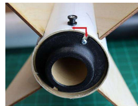
Figure 13-37: Slide Aft Ring to Fins (Top); Epoxy Outside of MMT (Top Center); Epoxy Inside of Airframe (Middle Center); Rail Button, T-Nuts and MMT Cap Installed (Bottom Center); Offset between T-Nut and Rail Button (Bottom)
