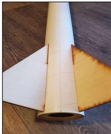
Figure 13-25: Measuring Fin Slots (Top); Measuring Half Way between Two Fin Slots (Top Center); Drawing a Line at the Half Way Mark on Tape (Center); Drawing the Half Way Mark on the Air Frame (Bottom Center); Markers to Indicate Rail Button Placement/Alignment (Bottom)
