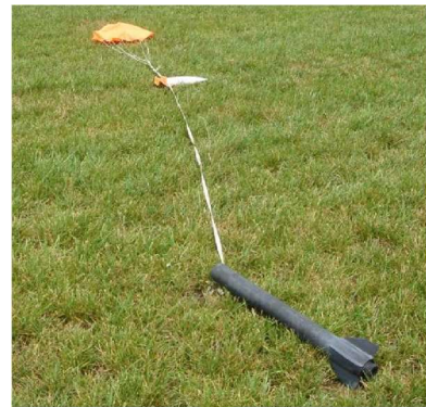
Figure 8-1: Single Event Recovery System
